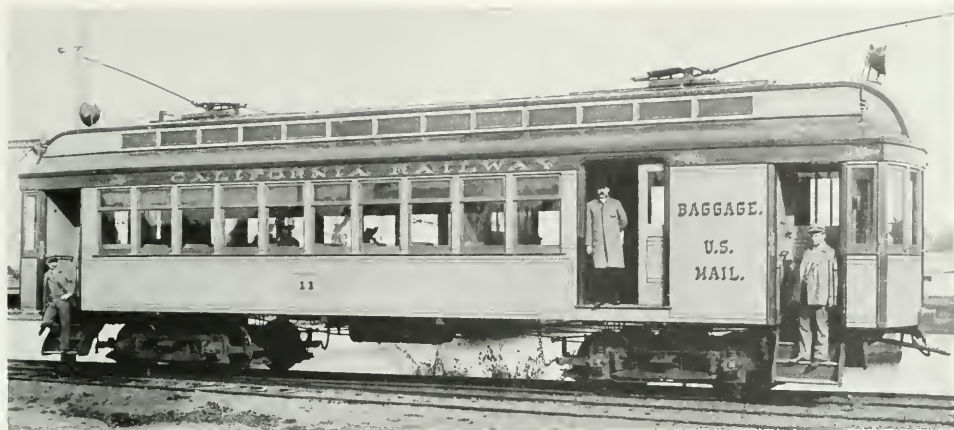
A Key System predecessor, California Railway, bought masterfully painted car 11 from Carter Brothers of Newark, Calif., in 1896. Its proportions and massive clerestory indicate a greater familiarity with steam car construction than with electric car building on the part of the local builder. INDUSTRIAL PHOTO SERVICE.
