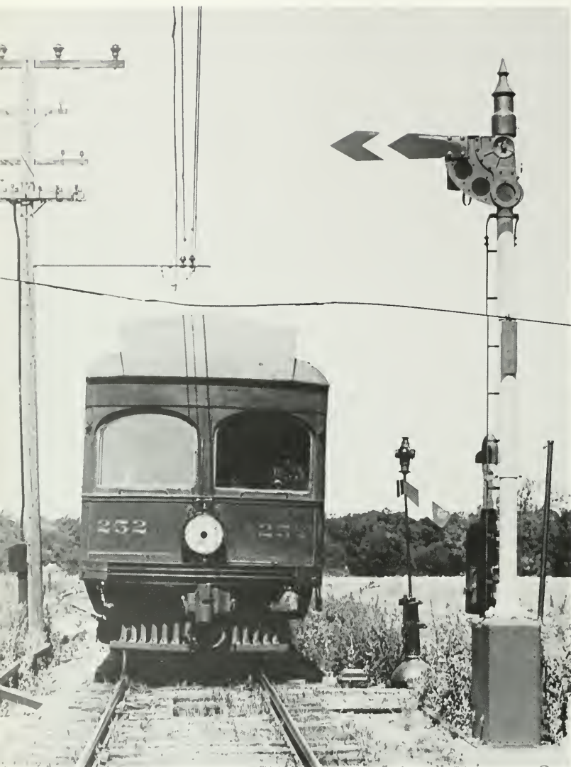
The crew of this Illinois Traction interurban viewed the roadbed from behind a truly generous expanse of plate glass. An early arrival in ITS ranks (American Car Company, 1904), car 252 predated the distinctive car design that soon became a virtual company trademark. WILLIAM D. MIDDLETON COLLECTION.
