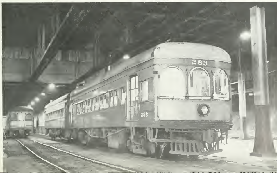
Workhorse combine 283, seen in the gloom of the St. Louis terminal in 1955, bore the unmistakable imprint of Illinois Traction electric car architecture, despite the blocked-off side window arches of a '30's rebuilding. Operation from the left-hand side was an unusual IT feature. The rectangular insert of safety glass in the motorman's window was a modern-day innovation. WILLIAM D. MIDDLETON.
