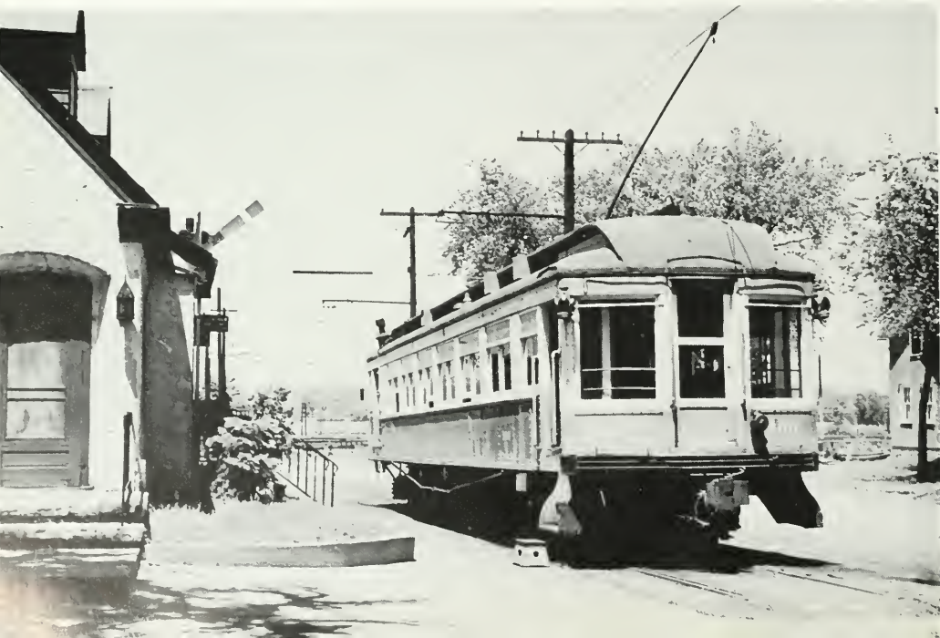
Rebuilt into a solarium-observation coach during the '20's, car 100 (at Cedar Rapids station) was the only member of WCF&N's trio of de luxe cars to survive a 1954 roundhouse fire that wiped out the road's shops in Waterloo. The 100 continued to operate in interurban passenger service until 1956. The unused semaphore alongside the station dated from the days when trains continued into downtown Cedar Rapids over city streets. WILLIAM D. MIDDLETON.
