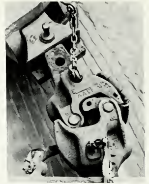
Illinois Terminal developed a special double-jointed coupling for company-owned box cars in order to make the curves on its line through Bloomington. Other interurbans used radial couplers, or employed slotted coupler knuckles and intermediate drawbars. HENRY J. McCORD.
