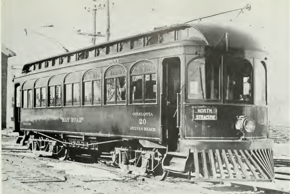
An otherwise conventional interurban of the Syracuse Northern Traction Company was distinguished by the experimental application of roller bearings. Several other interurbans, as early as 1910, made similar applications, far in advance of the adoption of roller bearings by steam railroads. ROBERT O. WATERS COLLECTION, FROM WILLIAM R. GORDON.
