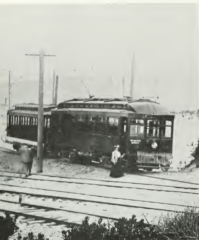
The Norfolk & Southern Railway, a steam road, operated a short interurban line from Norfolk to Cape Henry and the resorts of Virginia Beach. Combine No. 45, with an open trailer in tow, waited on the Virginia Beach wye about 1905. Gasoline rail buses took over the service in 1935. ALLAN H. BERNER COLLECTION.
