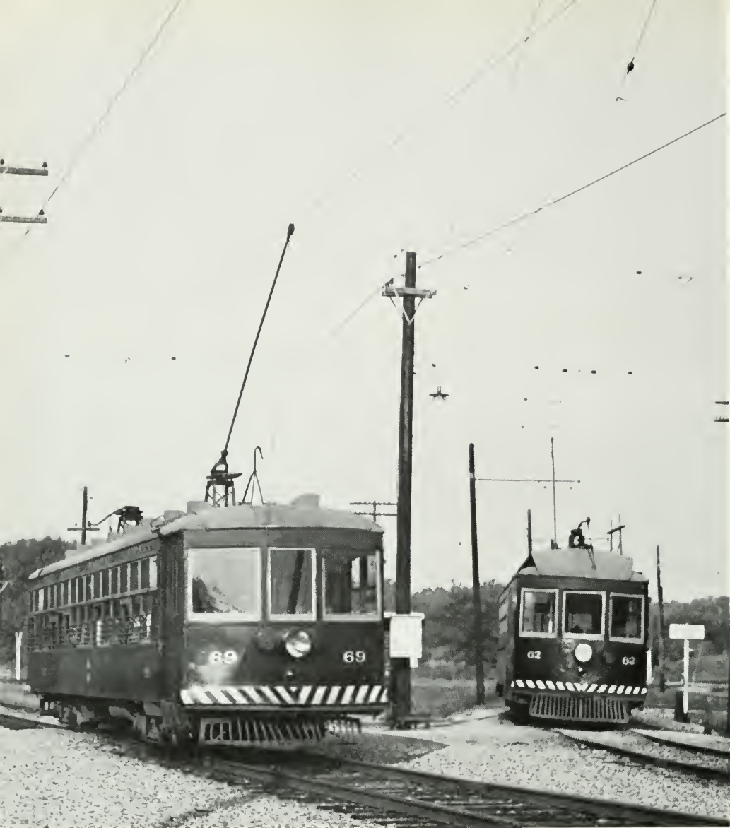
The Sand Springs Line began the replacement of its original heavy wooden equipment with secondhand lightweight cars during the '30's. Here, at Lake Station in 1946, are former Oklahoma Union Railway lightweight No. 69, en route from Tulsa to Sand Springs, and Tulsa-bound No. 62, one of the five lightweights acquired from the Cincinnati, Lawrenceburg & Aurora in 1934. Built by the Cincinnati Car Company in 1918, the CL&A cars were among the first lightweight cars built. GORDON LLOYD.
