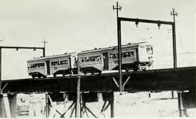
In the final years of its St. Louis-Granite City suburban service, Illinois Terminal provided streamlined PCC trolleys, modified for multiple-unit, double-end operation. A pair of them descended the St. Louis approach to McKinley Bridge in 1955. The Granite City cars, Illinois Terminal's last passenger operation, continued to run until 1958. WILLIAM D. MIDDLETON.
