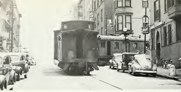
This scene on the Illinois Terminal at Bloomington, Ill., illustrates the difficulty encountered in handling freight around the streetcar curves found on interurban lines. HENRY J. McCORD.
