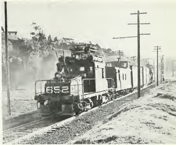
The bane of freight operations on the Sacramento Northern Railroad was the route over the Oakland hills, where grades up to 4 per cent were encountered. This southbound freight had successfully made the climb and was descending into Oakland late one afternoon in 1951. Pusher engine No. 652, a standard General Electric unit, had already dropped its pantograph. WILLIAM D. MIDDLETON.
