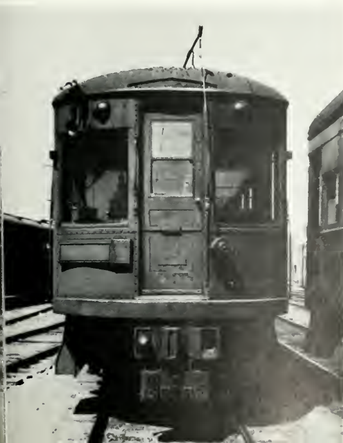
A close-up shows one type of fully automatic coupling, in interurban service on the Baltimore & Annapolis. WILLIAM D. MIDDLETON.
