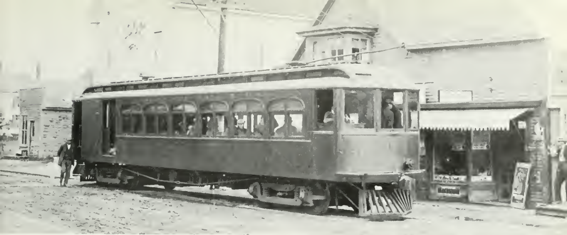
In 1913 the Wason works at Springfield, Mass., furnished a pair of cars that were more characteristic of Mid-western interurban practice than of New England. No. 70 is shown in front of the Odd Fellows Hall in Washburn. STEPHEN D. MAGUIRE COLLECTION.
