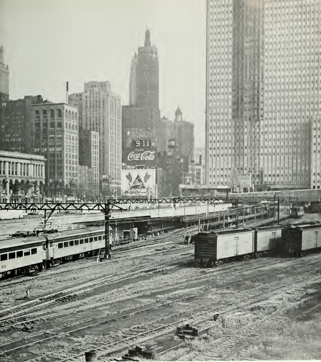
A South Shore Line express from Gary, Ind., slid into Illinois Central's Randolph Street Suburban Station in Chicago in 1955. Lengthened and fitted with picture windows, foam rubber seats, and air conditioning, this equipment helped place the South Shore in the forefront of passenger interurbans, but tonnage freight traffic moving behind heavy electric motive power had a lot more to do with the South Shore's continued prosperity in 1965. WILLIAM D. MIDDLETON.
