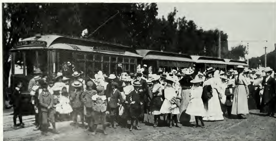
Both the Sixth and Main Street terminal building and the San Pedro interurban line were new when this photograph was taken about 1906. No. 279, scraping the pavement as it beeled into the terminal, was one of 130 semi-open cars delivered by the St. Louis Car Company between 1902 and 1906. The sidewalk semaphores and track switches were operated from the raised bay-window office to expedite heavy two-way movements in this then stub terminal, and to protect narrow-gauge city cars which also used Main Street's three-rail trackage. AL HAJI COLLECTION.
