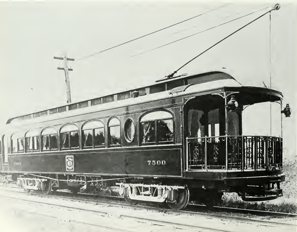
The company's glittering parlor car 7500, available for official duties or charter service, was fitted with deep solarium windows at the front end and this elegant observation platform at the rear. GEORGE KRAMBLES COLLECTION.
