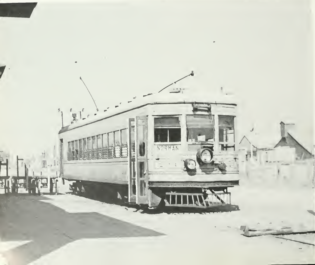
The Oklahoma Railway's steel combine Lindbergh was built for the company in 1917 by the St. Louis Car Company. Scrollwork painting and the glass in the lower panels of the baggage door augmented the "de luxe" appearance lent by white tires. O. F. LEE COLLECTION.
