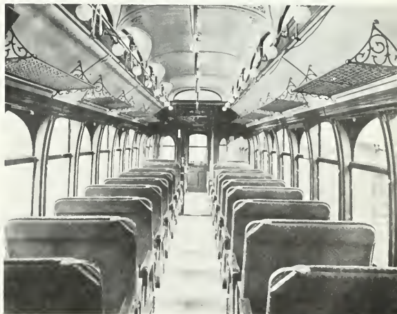
Interior appointments of this car, built by Brill in 1907 for the West Shore Railroad's Utica-Syracuse electrification, were typical of the early interurbans. The walkover seats were upholstered in figured plush, and the interior was finished in inlaid mahogany. The carbuilder's fanciful decorative touch was evident in the embellishments applied to the full Empire ceiling and the elaborate baggage racks. INDUSTRIAL PHOTO SERVICE.
