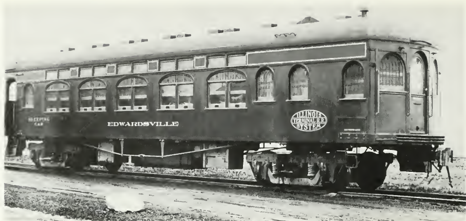
The interurban sleeping cars introduced by Illinois Traction in 1910 featured such advantages as upper-berth windows, extra-long berths, and individual safety deposit boxes. The Edwardsville was built by the St. Louis Car Company in 1913. WILLIAM J. CLOUSER COLLECTION.
