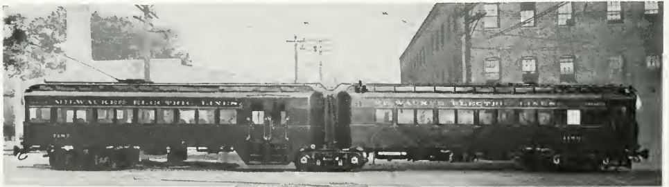
To provide increased seating capacity in a single unit, a few lines came up with articulated interurbans. The Milwaukee Electric Lines created eight of them in its Cold Spring shops in 1929 from conventional steel cars acquired from the Indianapolis & Cincinnati Traction Company. The resulting "duplex" units seated 84 passengers. STATE HISTORICAL SOCIETY OF WISCONSIN.
