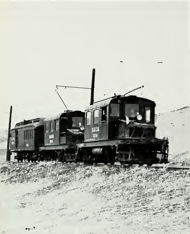
Trailing a former Colorado & Southern combine which served as a caboose, a pair of D&M narrow-gauge steeple-cab locomotives ran M.U. near Leyden in 1950. The unusual engines were leased from Denver Tramways. Freight equipment was painted a simple black, but passenger cars were the same golden yellow as DT streetcars. ROSS B. GRENARD JR.
