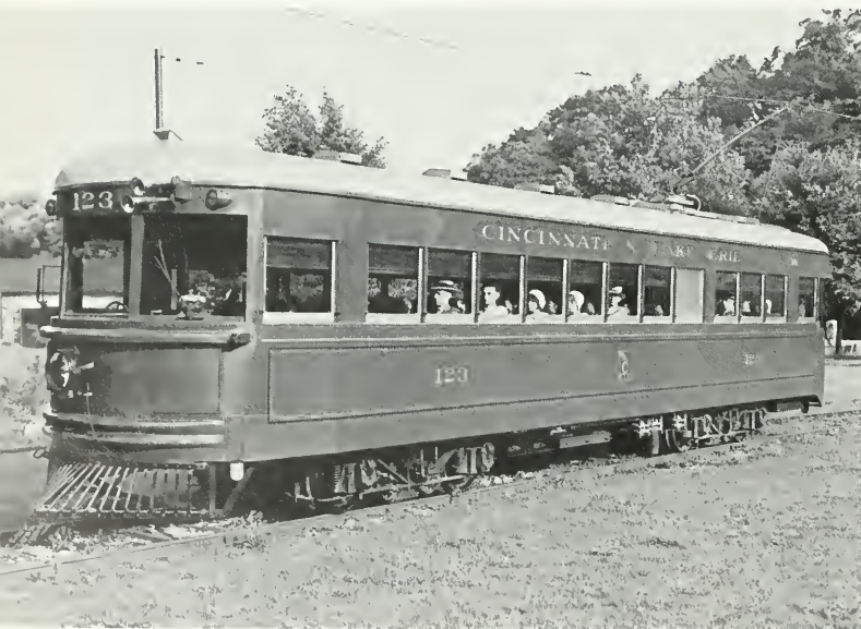
Exhaustive testing produced the phenomenal "Red Devil" lightweight, high-speed car for the Cincinnati & Lake Erie in 1930. Ten were built as straight coaches, and 10 as coach-lounges, fitted with swank furniture and provided with "wrap-around" windshield visibility from the observation section. The 123 was photographed at Moraine Park. BOTH PHOTOS: MAYFIELD PHOTOS INC.
