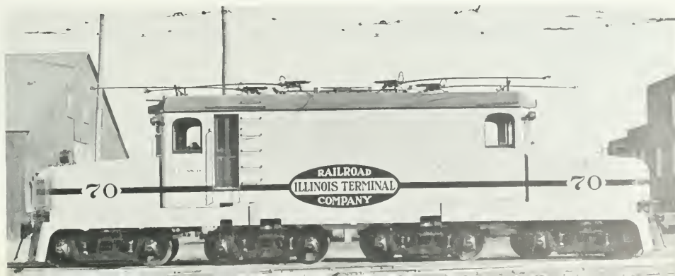
Last in a long line of home-built Illinois Terminal electric motive power were five of these 16-wheeled Class D locomotives upgraded by Decatur shops between 1940 and 1942. They weighed 108 tons and were equipped with eight traction motors totaling 1800 horsepower.
