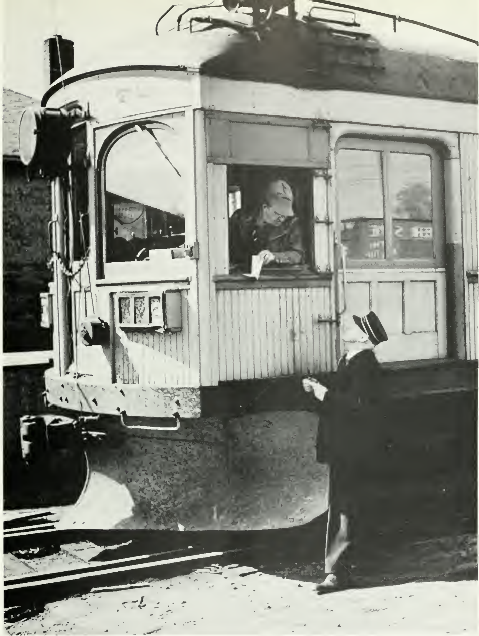
In the earlier years of the interurban era, two-man crews of motorman and conductor were almost universal, and sometimes interurban lines patterned their operating rules after those of steam railroading. Among these was Iowa's Fort Dodge Line, which even as late as 1955 still went about the job of running electric cars in the traditional manner. Here conductor F. E. Nunamaker passes up a clearance card from the operator at Fort Dodge to motorman E. J. Berg before their departure with southbound train No. 2 for Des Moines. Both wore the respective blue serge uniform and overalls of their occupations. WILLIAM D. MIDDLETON.
