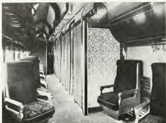
The Holland Palace Car Company hoped to revolutionize the long-distance interurban business with a combination design that converted from parlor to sleeping car through the use of rolling partitions. Only two of them were ever built. STEPHEN D. MAGUIRE COLLECTION (ABOVE); GEORGE KRAMBLES COLLECTION (RIGHT).
