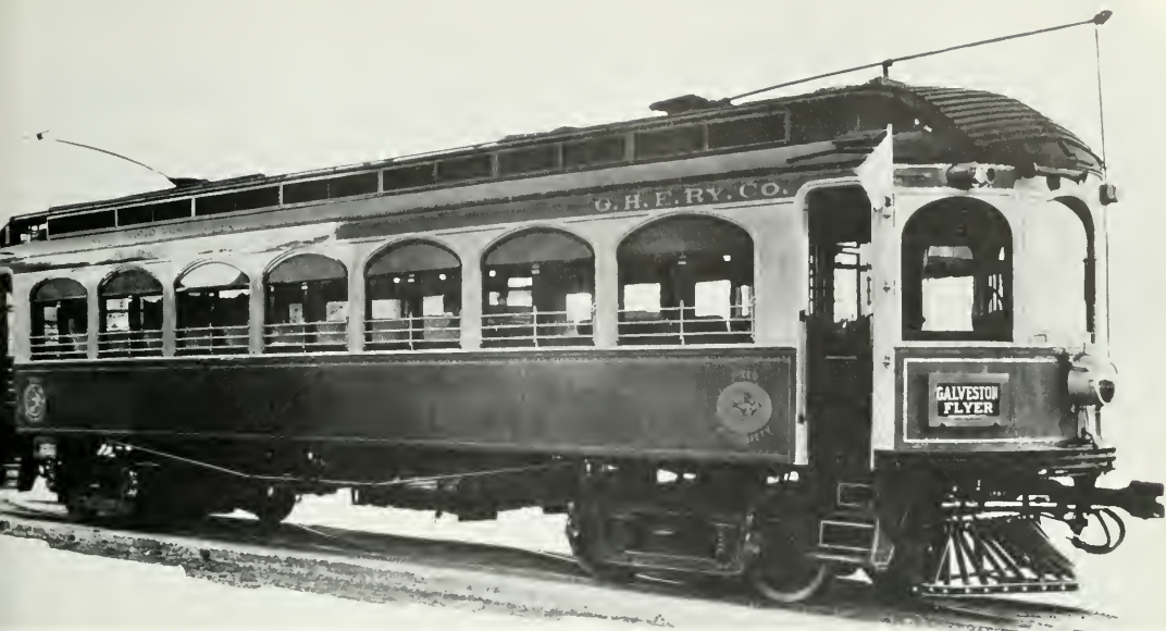
The zenith of wooden interurban car architecture was represented by the equipment delivered in 1911 by the Cincinnati Car Company for the Stone & Webster Engineering Corporation's Galveston-Houston Electric Railway. This car is seen in the blue and white "bluebird" colors worn during the '20's, when the Galveston Flyer won honors as America's fastest interurban. GEORGE KRAMBLES COLLECTION.
