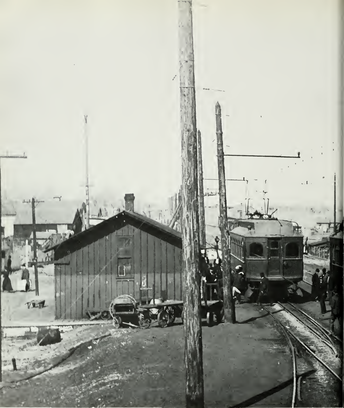
Between Denver and D&E Junction, a distance of some 16 miles, Colorado & Southern deemed it advisable to construct a new and separate line for its electric subsidiary, but the remainder of the distance to Boulder was operated over either of two C&S steam lines which had been electrified for the interurban service. This activity at Louisville about 1910 indicates the close integration of D&E
