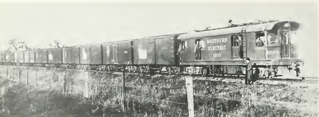
At the time of its construction by Northern Electric's Chico (Calif.) shops in 1911, 82-ton No. 1010 was said to be the largest and heaviest interurban locomotive in the West. All electrical equipment was carried beneath the floor and the elongated body provided space for l.c.l. freight. In 1930 NE's successor Sacramento Northern rebuilt the big locomotive along more conventional lines. WESTERN PACIFIC RAILROAD.
