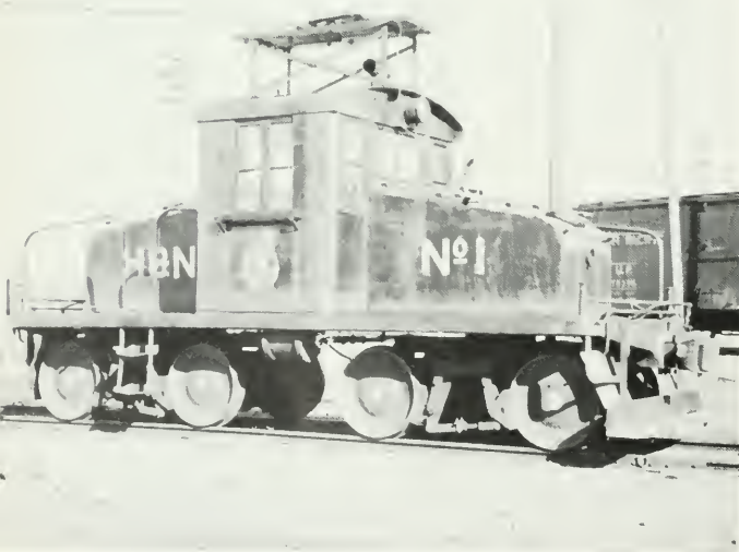
This unusual General Electric locomotive, operated on the Hutchinson & Northern in Kansas, was equipped with a "frameless truck." Axle bearings were placed in an extra-heavy traction motor frame, which was provided with lugs over the bearings to receive the equalizer bars. FRED FELLOW.
