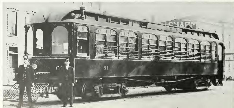
This Northern Ohio Traction & Light Company interurban was constructed with the "Washington" sash, an arrangement which employed clear glass upper sash for improved interior illumination but retained the class of "Gothic" window design with dummy art glass arches in place of the customary letter board. O. F. LEE COLLECTION.
