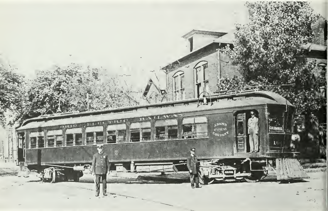
Flanges squealed as this Ohio Electric wood combine negotiated abrupt track curvature in the streets of Zanesville, O. The car was characteristic of hundreds of its contemporaries on the interurban properties of the Midwestern states. STEPHEN D. MAGUIRE COLLECTION.
